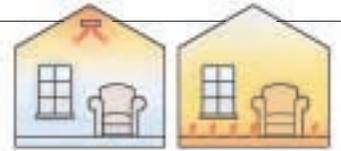
*In forced air homes, overheated air rises to the ceiling leaving the level near the floor, where the people are, too cool. But, in a Warmboard home, it's just the opposite. The people are comfortable and the ceiling temperatures are reduced.*
