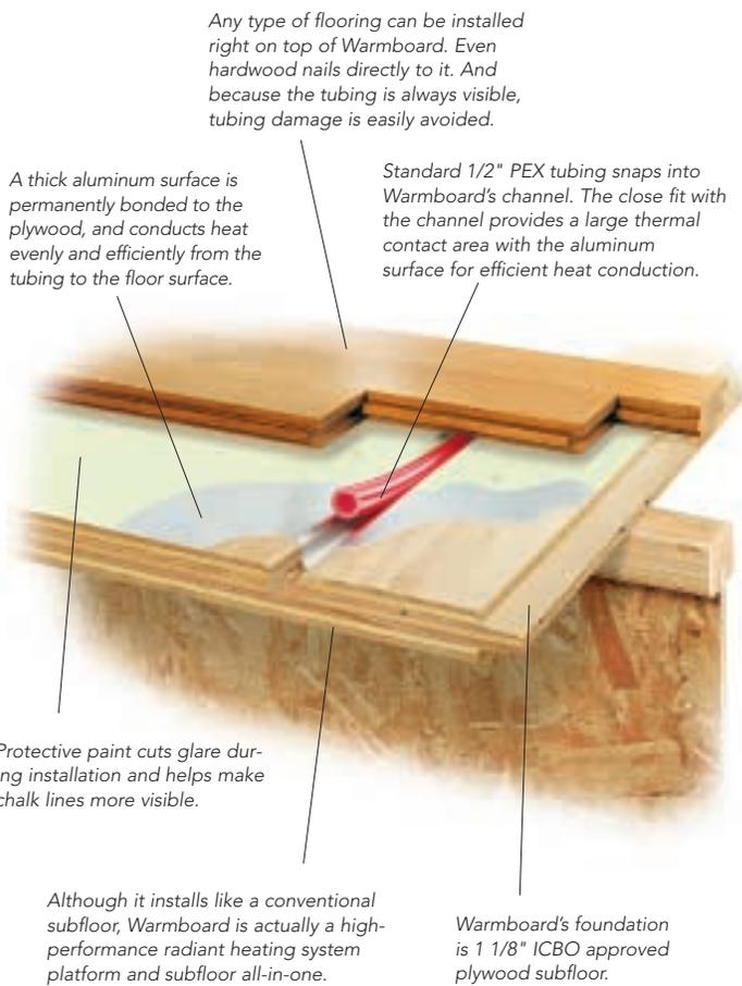
*Any type of flooring can be installed right on top of Warmboard. Even hardwood nails directly to it. And because the tubing is always visible, tubing damage is easily avoided.*
